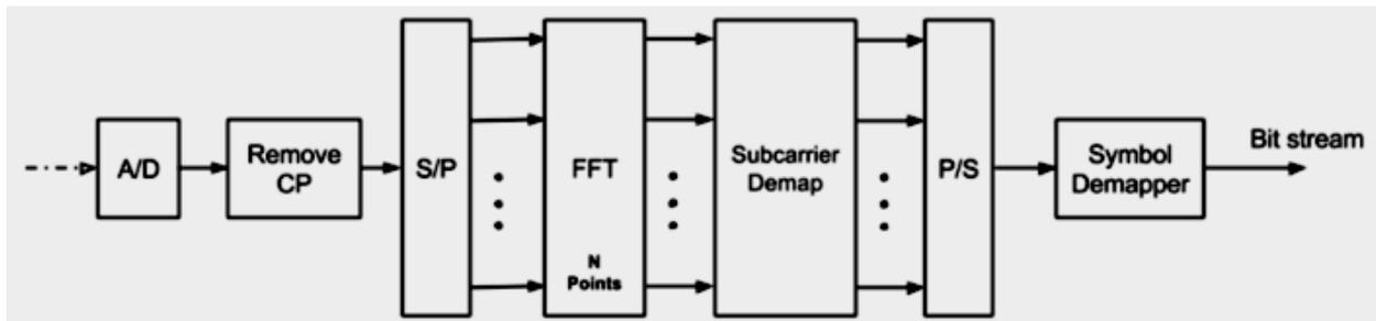
Figure 2.2 OFDM scheme for receiver.
