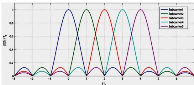
Figure 1.1 Orthogonal subcarriers.
