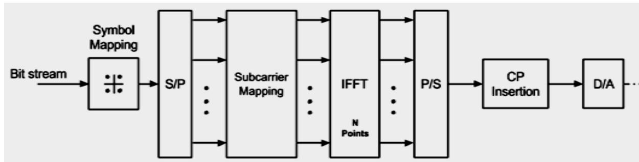
Figure 2.1 OFDM scheme for transmitter.
