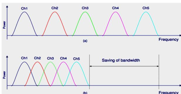
Figure 2.1 Comparison between conventional FDM and OFDM.
