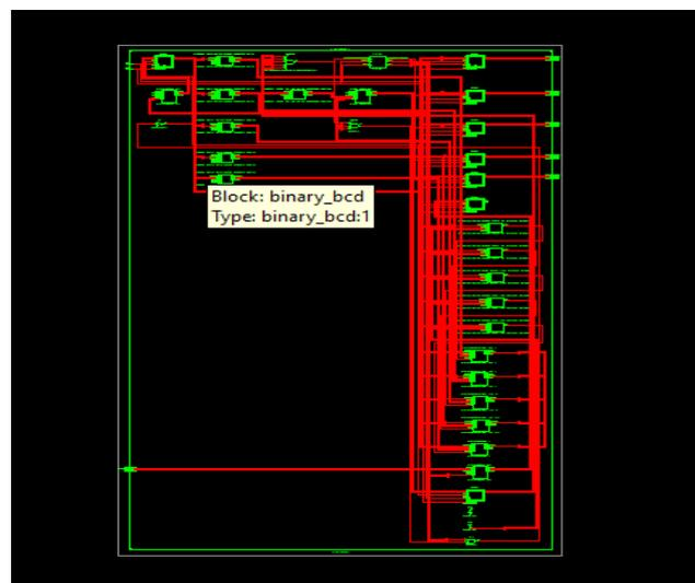
Fig. 5. RTL View of 16 bit Binary coded decimal Converter
