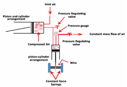
Figure 2 : Block diagram of the PCS system along with the compressor
