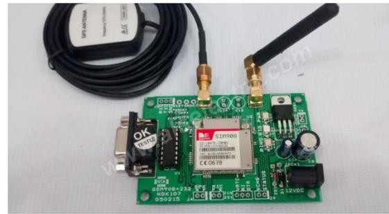
**Fig 3 GSM Module**
