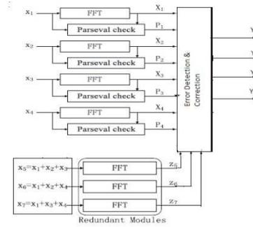
Fig 2.1 Parallel correction method
