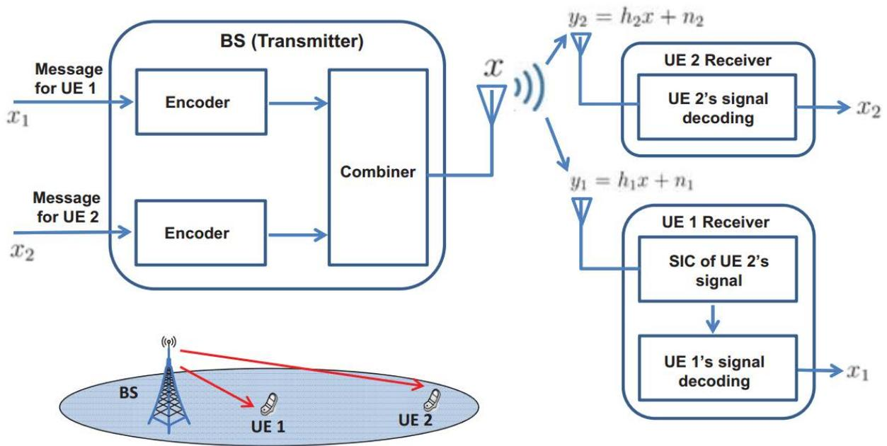
Figure 2.1 superposition coding and SIC receiver.
