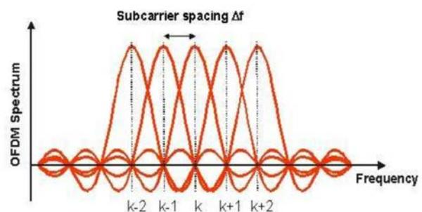
Figure 1.1 Orthogonal Frequency Division Multiplexing Spectrum
