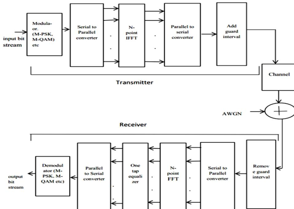
Figure 2.1 OFDM system model
