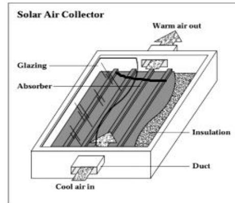
Fig. 1 Solar air collector
