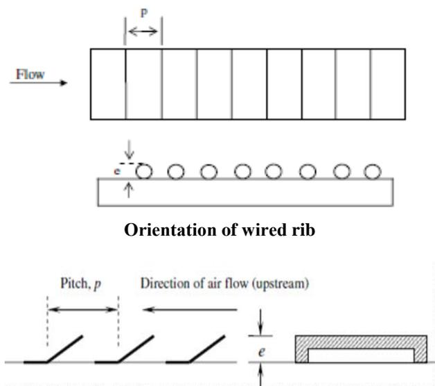
Fig. 2 Orientation of Inverted U shape rib
