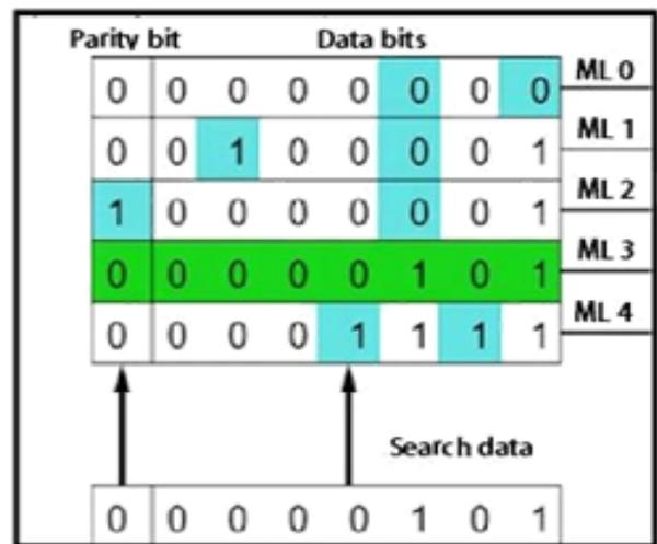
Figure 5. Search Speed Boosting With a Parity Bit
