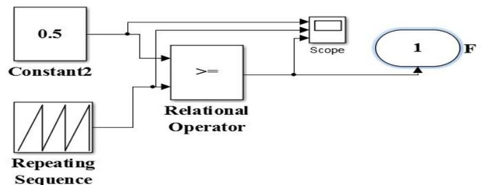
Figure 7 PWM logic matlab simulation
