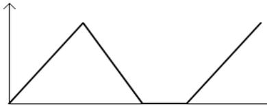
Figure 6 Discontinuous conduction modes
