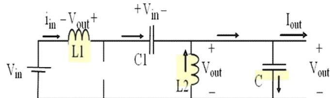
Figure 4 basic sepic converters OFF state
