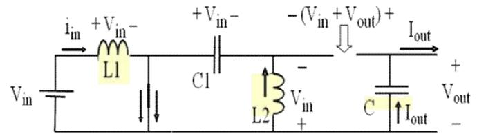
supplies energy to the inductor (L1), capacitor (C1). Voltage across the inductor (L2) during capacitor (C1) is discharging. Voltage across output  $V_{out}$  is give capacitor (C) in this time capacitor (C) also discharge. Apply KVL  $V_{L1} = V_{C1} = V_{in}$ .
