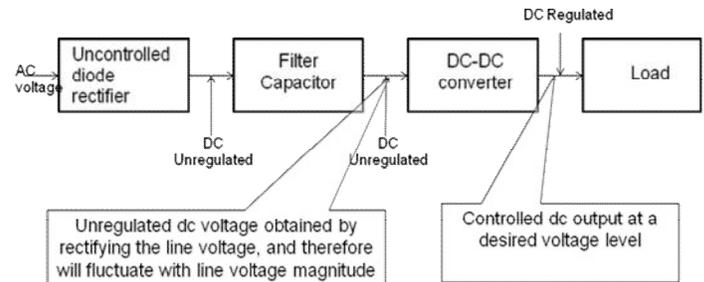
Figure 1 basic block diagram of DC-DC converter
