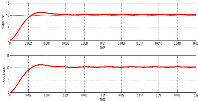
Figure 8 Open-Loop SEPIC Converter Response for  $V_{in}=10V$
