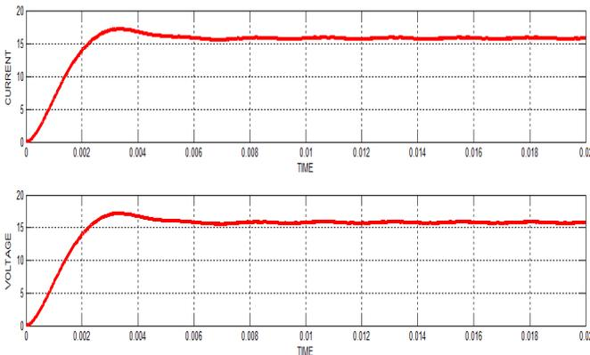
Figure 9 Open-Loop SEPIC Converter Response for  $V_{in}=15V$
