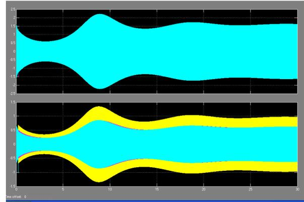
Fig.2.4.1 Induction generator terminal Voltage  $V_L$ , and line current  $I_L$
