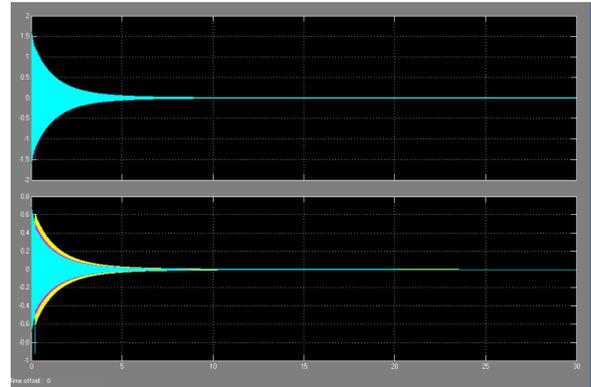
Fig. 2.2.1 Induction generator terminal Voltage  $V_L$ , and line current  $I_L$
