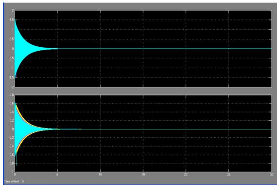
Fig. 2.1.1 Induction generator terminal Voltage  $V_L$ , and line current  $I_L$
