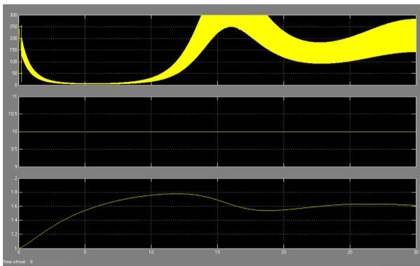
Fig. 2.3.2 Power in kw, wind speed in m/s and induction generator speed in p.u.
