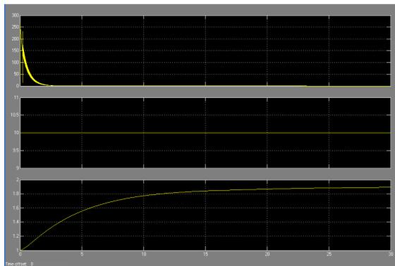
Fig. 2.1.2 Power in kw, wind speed in m/s and induction generator speed in p.u.
