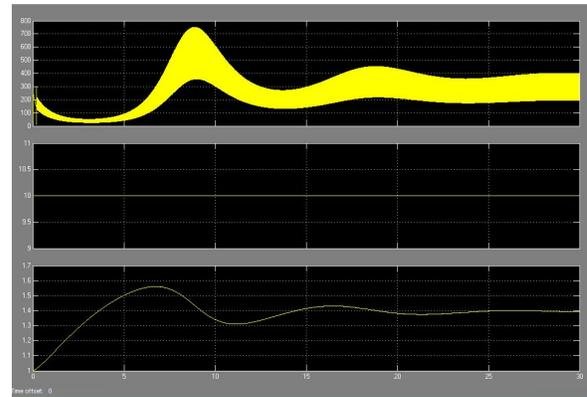
Fig.2.4.2 Power in kw, wind speed in m/s and induction generator speed in p.u.
