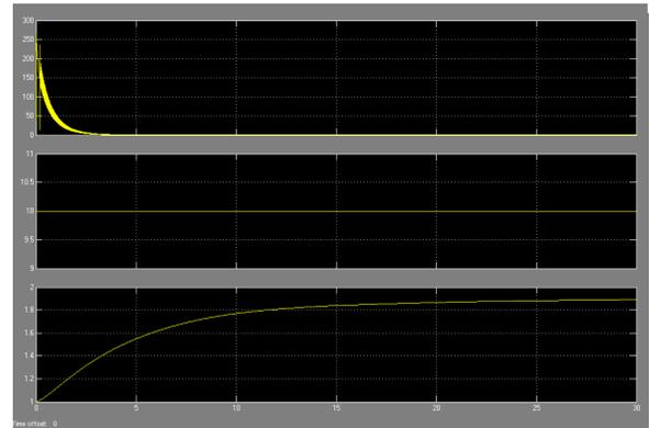
Fig.2.2.2 Power in kw, wind speed in m/s and induction generator speed in p.u.
