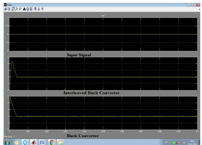
Fig. 5.6 Comparative resultant wave form of Buck Converter and Interleaved Buck Converter
