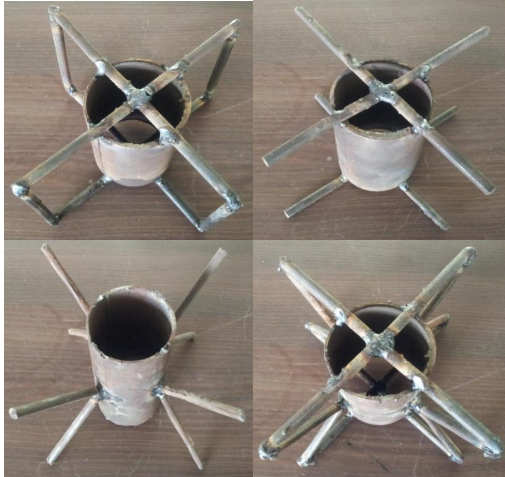
Fig. 3. Different Reinforcement Used Namely B, K, X & Σ Respectively
