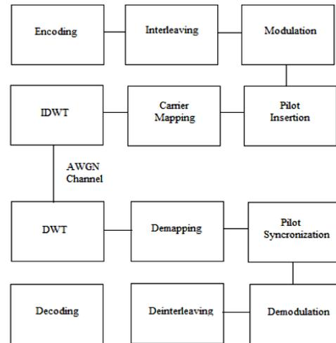
Fig .4: Wavelet based OFDM system design
