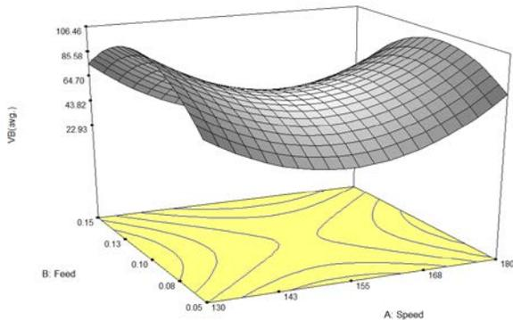
Figure 3 Effect of cutting speed and feed rate on flank wear (depth of cut 0.25mm.)
