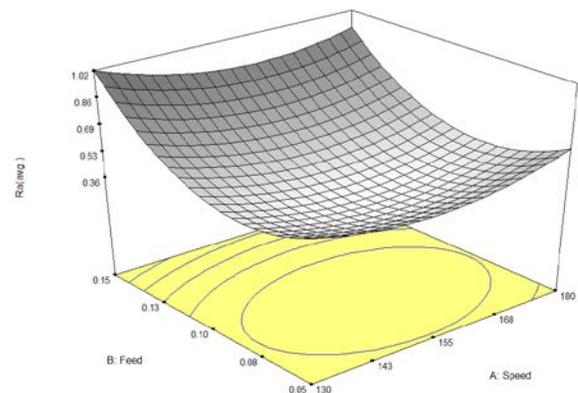
Figure 5 Effect of cutting speed and feed rate on surface roughness
