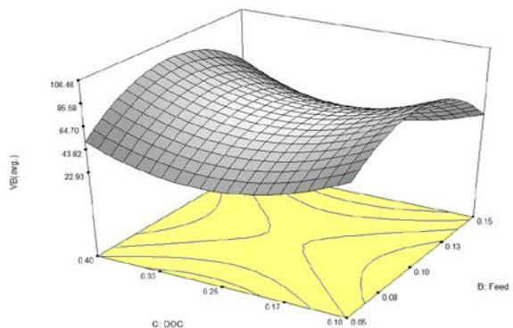
Figure 4 Effect of depth of cut and speed on flank wear
