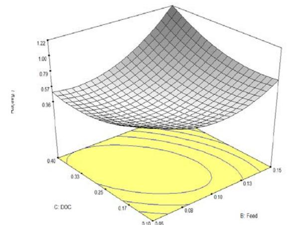
Figure 6 Effect of depth of cut and feed on surface roughness
