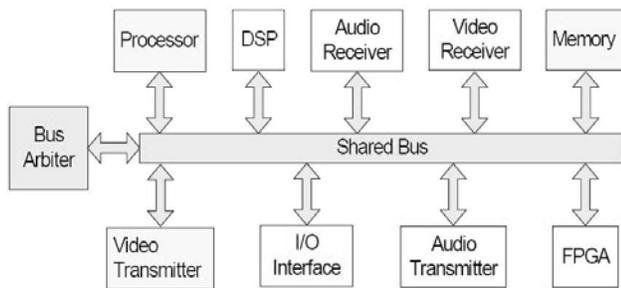
Fig. 1.2 Shared Bus System for SoC
