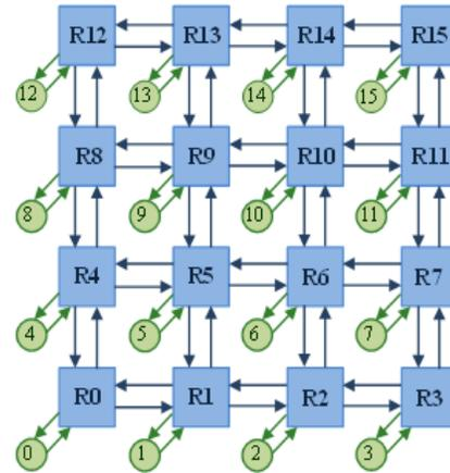
Fig. 2.1 4x4 Mesh Architecture
