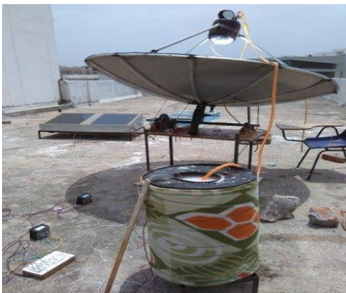
fig. 1. Experimental set up of parabolic solar collector
