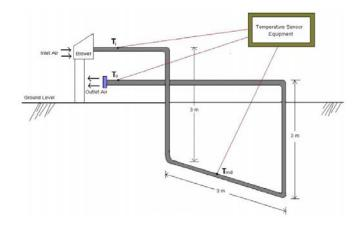
Three pipe each length of 3 m are connected in Series connection, made up of GI pipes and buried at a depth of 3 m in a flat land with dry soil. The Series connection of GI pipes exhaust manifold for air passage. Ambient air was sucked through the pipe by means of a centrifugal blower by a 2 phase, 0.25 hp, 230 V and 2800 rpm motor.
