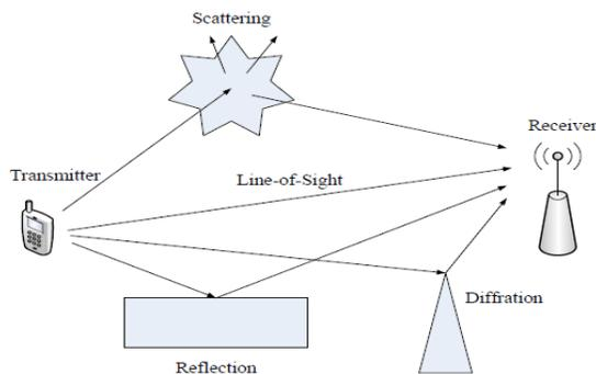
Fig. 3 Example of a wireless channel in which there are multiple propagation paths between the transmitter and receiver.
