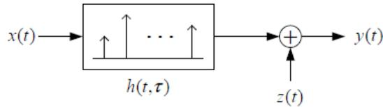
Fig. 4 Channel model in a wireless communication system.
