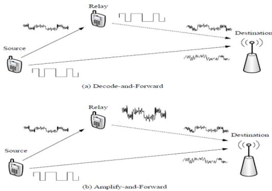
Fig. 6 Amplify-and-Forward and Decode-and-Forward signal
