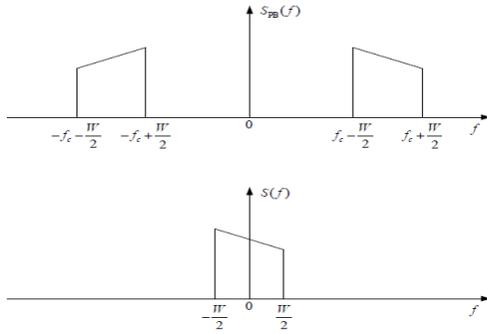
Fig. 2 The relationship between pass-band spectrum  $SPB(f)$  and its equivalent baseband spectrum  $S(f)$ .
