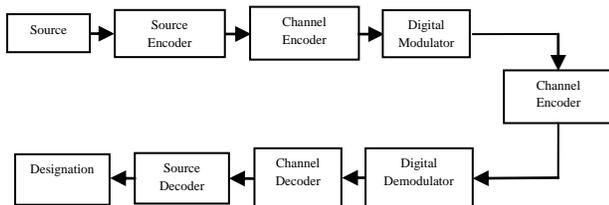
Fig. 1 Basic elements of a digital communication system.
