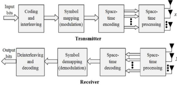
Fig.2: MIMO Transmit and Receive System Block Diagram.
