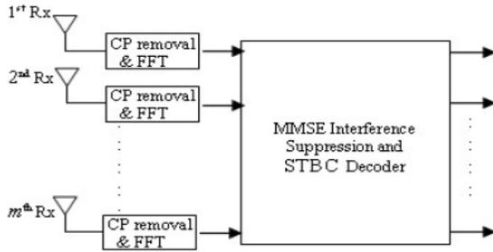
Fig.6. Space-time block coded MIMO-OFDM receiver
