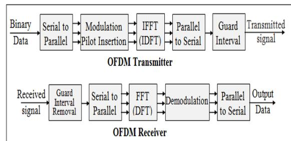
Fig. 4: OFDM Transmit and Receive System Block Diagram.
