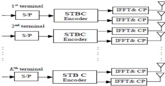
Fig. 5: Space-time block coded MIMO-OFDM transmitter
