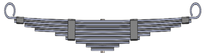
Fig.2.Steel with Heterogeneous Concept of leaf spring Assembly
