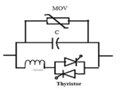
Fig 4.1 Thyristor controlled series capacitor
