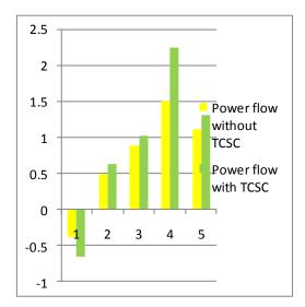
Fig 5.2 Power flow with and without TCSC
