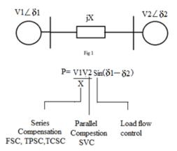
Fig 2.1 Active power transmission equation
