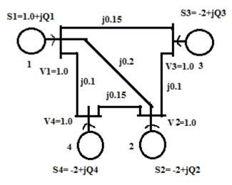
Fig 5.1 IEEE 4 bus test system
